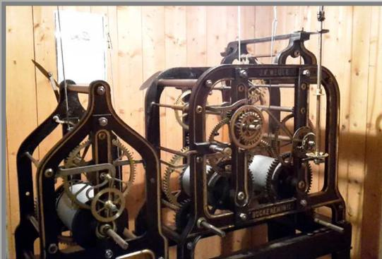
Turret clock with clockwork which is wined up once a week with a hand crank. You may hear the ticking if it is quiet in the steeple hall. The hands on the dial show a small difference of two minutes due to the wearing of the old gear wheels. New ones are unfortunately not available.
